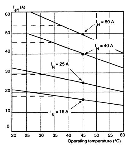
Current derating curves as a function of ambient temperature (IN = nominal current at 45°C)
