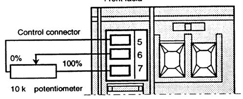
External potentiometer wiring example (view from below)
