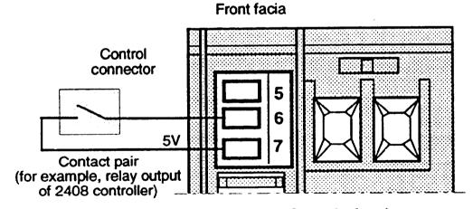
Control contact wiring example (view from below)
