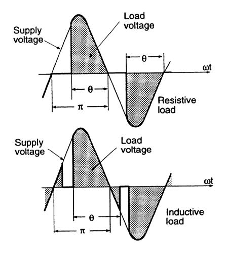
Load voltage in 'phase angle' firing mode (θ: thyristor firing angle)
